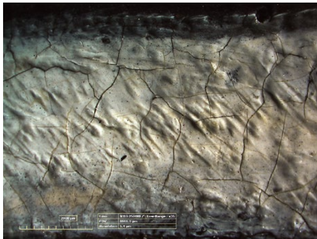
Fig. 22 Cat. no. 5, microscopic image of the paint surface with raking light angle at 35x magnification using Hirox digital microscope. Image Redivivus
